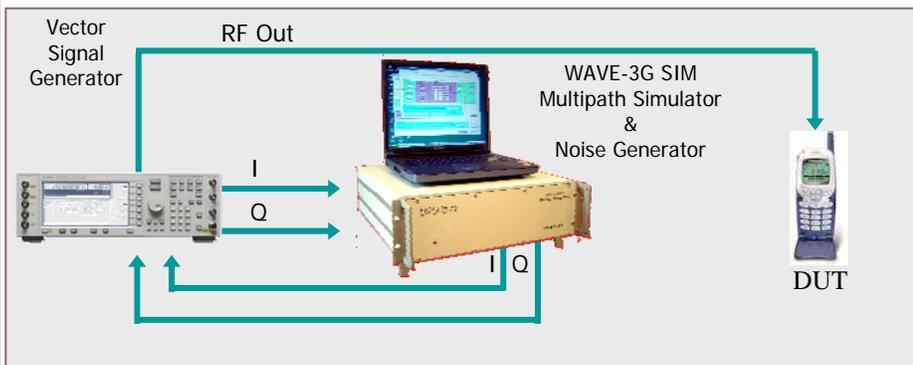
Combining WAVE-3G SIM with a Base Station Emulator and Vector Signal Generator yields a powerful and comprehensive 3G mobile test solution. Since a digital power meter enables accurate and repeatable C/N settings even with multipath faded signals, your FER or BLER measurement confidence level is high. This allows shorter test times and better design decisions.
